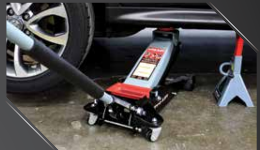
*Support load with a pair of Jack Stands
